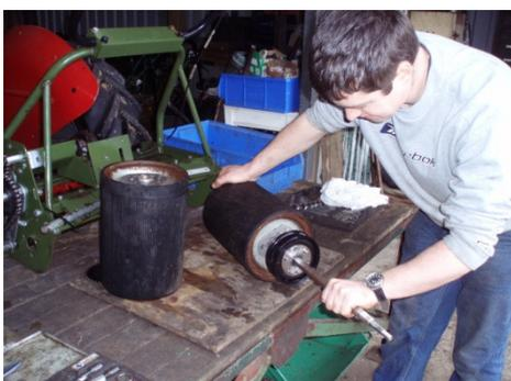
The condition of the rear-rollers rubber coating (on the Royale and Webb 24) is inspected closely. Replacement roller sections (with undamaged coating) are fitted
