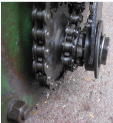
We fit new and unworn ratchet/sprockets, which will last for many decades with basic maintenance
